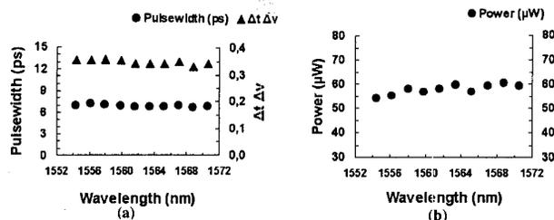
Fig. 3. (a) Variation of the pulsewidth and pulsewidth-bandwidth product vs wavelength, (b) Variation of the output power vs wavelength.
